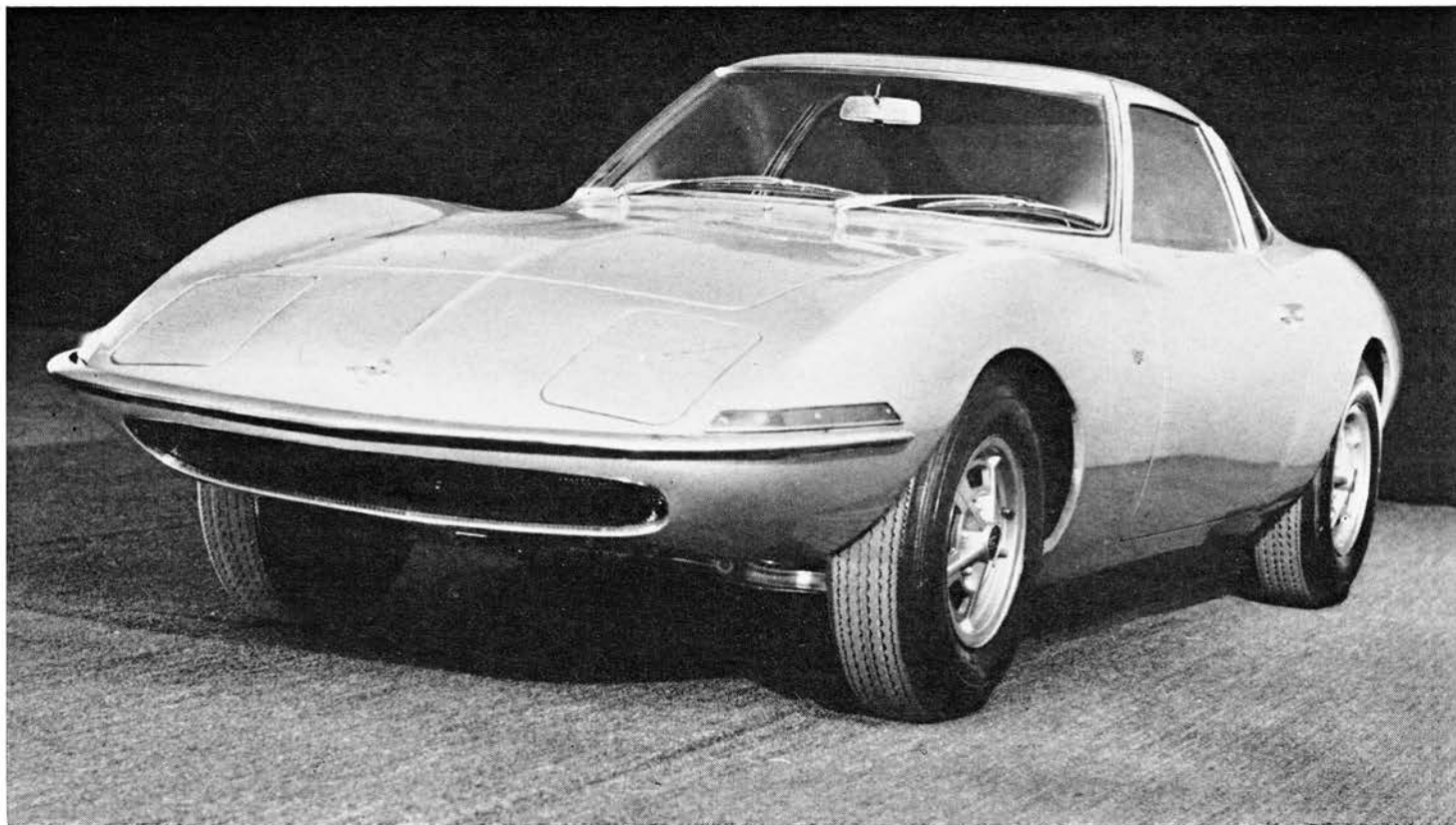
OPEL'S EXPERIMENTAL GT is built on the Kadett floor pan and uses the Kadett independent front suspension. Its engine is the Opel 1897-cc (106 cid) sohc four, modified to produce 108 DIN bhp; up from 90 stock.
