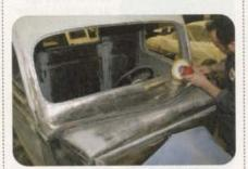
The top of the cowl was next on the list; every bit of surface rust was ground away. The weld area where the original cowl vent was located was ground smooth as a baby's behind.
