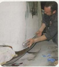
The long sanding board allows John to work from the cab's rear corner forward to the cowl. The continuous surface will likely be better than when the truck was brand new. Notice the amount of material on the floor.
