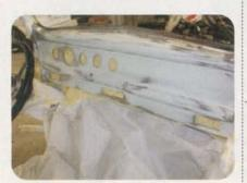
With filler on the dash panel and the added lower A/C panel, the dash is beginning to look much more integrated. We think the Classic Instruments analog gauges and the backlit Vintage Air A/C controls will look great, and very sanitary next to the unified dash surfaces.
