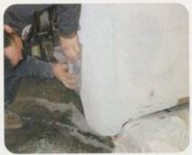
John works the cab's rear corner surface with a sanding block — again moving in an X-pattern for the most part. The bottom of the cab's corner has an inner and an outer wall. When the cab was restored, the corner was sealed with metal to prevent moisture from entering between the inner and outer surface.
