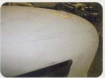
This image of the rear roof panel shows a surface change or seam between the top and the rear of the roof. We agreed that this detail was important to retain to prevent the transition of the roof from looking too soft.
