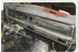
The dash will also be primed and painted body color – it needed to be prepared also. At least we've eliminated the unwanted holes in the dash and have fresh metal where the Classic Instruments gauges will be mounted flush to the dash panel.
