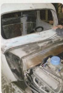
Important Tip: A concave surface is best worked with a curved surface tool, such as a rolled sanding pad. John uses a cardboard paper roll with sandpaper added. The sanding motion is still primarily in an X-pattern.
