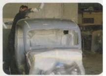
The crew cleaned with SHER-WILL-CLEAN® Solvent Cleaner — these products are also available: R7K156; AQUA-MATE™ Low VOC Surface Cleaner W4K157 or UltraClean® Surface Cleaner R7K158. Simply wipe dry with a clean, dry cloth. Alfred applied two or three medium coats of ULTRA-FILL for a very sandable surface. Complete instructions can be found on the Internet as well as on the can.
