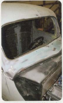
The top of the cowl was worked in several thin layers. This area is one of the few with a "fillet" or concave surface.
