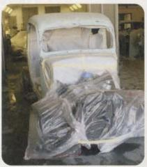
Brea Hills' crew taped off the engine and the rear of the chassis to prevent what little overspray was in the air from floating onto unwanted surfaces. The HVLP spray guns put much less material into the air than paint guns from a decade ago.
