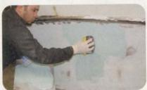
John uses a squeegee to apply the filler in uniformly thin coats on the rear panel. Notice that he is wearing rubber gloves for protection. One goal before catalyzed filler was applied to the rear panel was to keep the large surface from oil-canning (moving in or out). This was important to ensure that the filler material won't crack, and that the eventual topcoat will not be damaged as a result.
