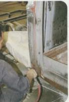
John moves to the passenger side of the cab, cleaning old filler and primer. We will extensively clean the inner floor and seat riser in the near future to prevent rust from attacking the interior metal surfaces.
