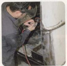
John cleans the restored rear corners of the cab and the door jambs with an air-powered rotary tool.
