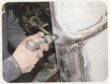
Important Tip: A wire brush on the rotary tool is good for thoroughly cleaning the tightly curved surface of the cab's body reveal.
