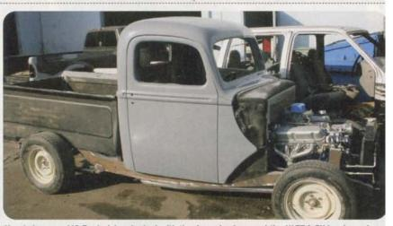
Here's how our '40 Ford pickup looked with the doors back on and the ULTRA-FILL primer dry. Our next goal is to assemble the front fenders, hood and grille. We didn't primer these items in the event that they may need some further adjustment in order to fit the cowl and hood. More good construction tips for 1940 Ford owners to come — stay tuned!
