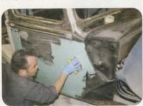
John works the passenger side door skin and the side of the cowl at the same time to create a continuous surface through the two panels.
