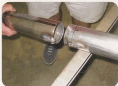
Felt tip markers show how the parts are aligned on the exhaust tubing, and they help Ed identify left from right and front to rear when he assembles all of the individual parts. You might consider a letter punch to identify parts after they're coated or plated.
