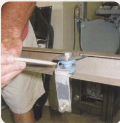
The rubber grommets have a male side and a female side that are neatly connected to make pairing them a cinch.
