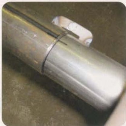
One neat feature is this small flange that Ed welded to the extension, a small bolt and nut to keep the tailpipe extension securely located.
