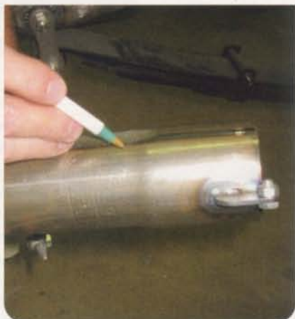
Notice how the diameter of the tailpipe extension is opened up slightly to slip over a section to the rear portion of the exhaust tubing. This service can be obtained from a muffler shop for a nominal fee.
