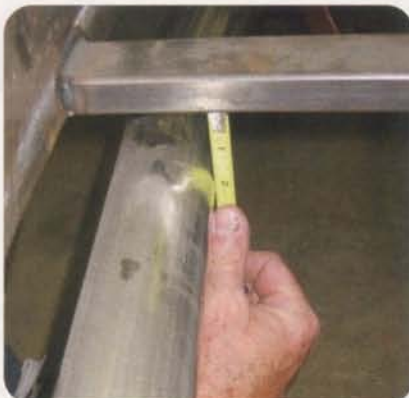
Clearance is checked over and over to ensure that no part will touch the frame rail or cross members.
