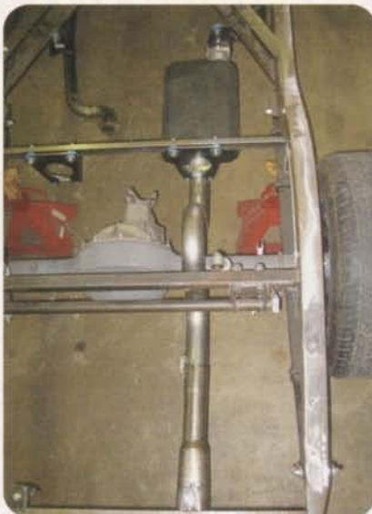
The passenger's side of the exhaust system is nearly complete. Notice that the tubing goes over the rear axle and passes under the fuel tank with adequate clearance.
