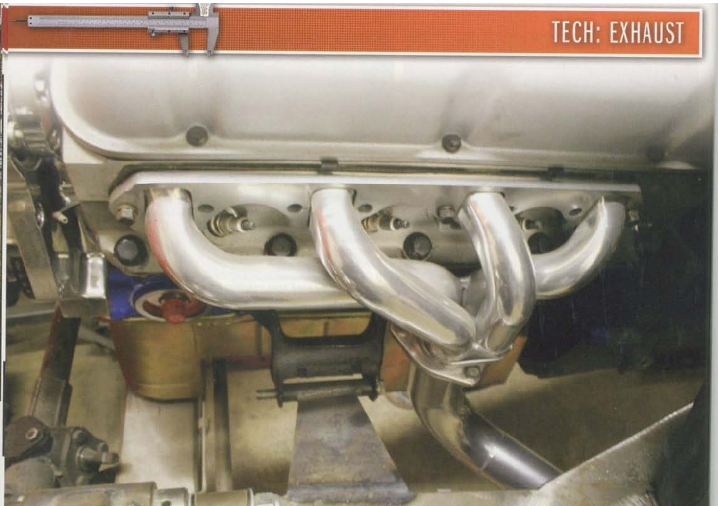
A good exhaust system begins with a tubular header that can pass between the frame rails and avoid the motor mounts. This Sanderson shorty header came in bare steel, but it was covered with a high performance coating to prevent discoloration and rust.
