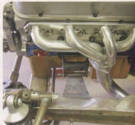
A high performance coating (HPC) is a great investment in a good-looking exhaust system that will last the life of the vehicle and increase the value of it as well. These coatings are typically sprayed on and then baked in an oven at high temperatures for a tough finish that resists coloring and rust.
