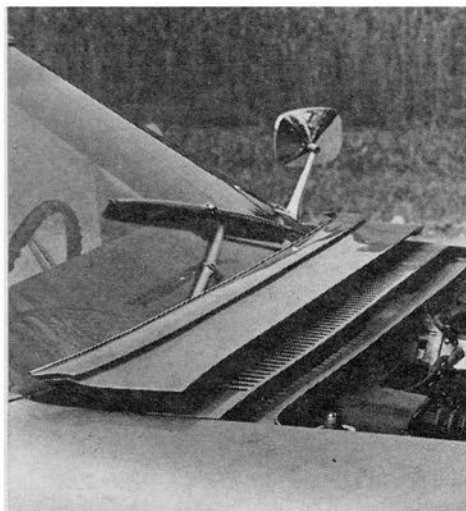
RETRACTABLE windshield wiper arms are concealed by sliding panel.
