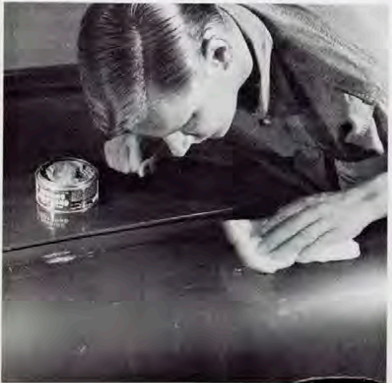
Below left: Minor scratches and surface scrapes can be buffed with rubbing compound if blemish isn't all the way through to body. Rub carefully and just enough to remove scratch.
