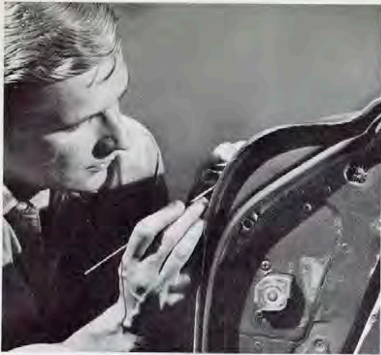
Above left: Take care of door-edge nicks with a fine camel hair brush as shown. Sand the chipped edges lightly with #400 sandpaper and brush paint on lightly.
