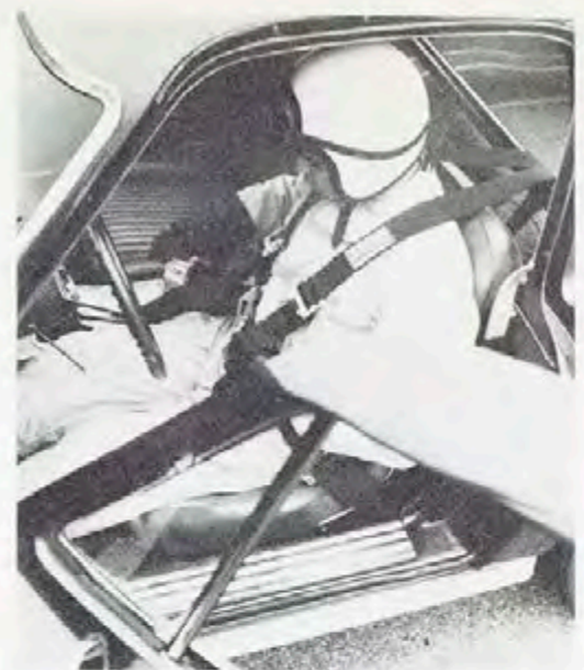
Above left/ Bill Kane straps himself into a test Corvette with special shoulder harness in addition to the regular seat belt. Above right/ Instrumented brake test car with huge dial for easy reading. Below/ Brake test car going through its paces.
