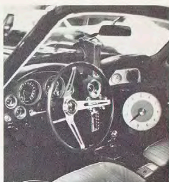
Above left/ Bill Kane straps himself into a test Corvette with special shoulder harness in addition to the regular seat belt. Above right/ Instrumented brake test car with huge dial for easy reading. Below/ Brake test car going through its paces.
