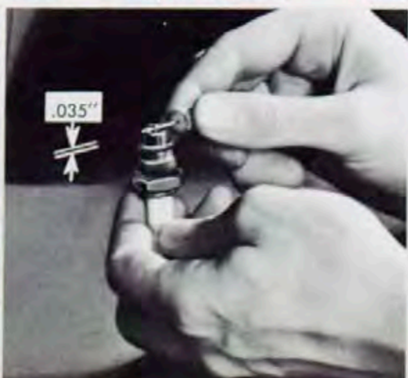
1. Install spark plugs with a torque wrench for proper tightness. 2. Always gap plugs identically. 3. Cutaway of typical spark plug showing gap for normal driving.
