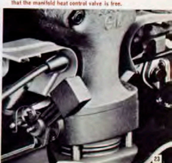
M. On carbureted engines, always check to see that the manifold heat control valve is free.
