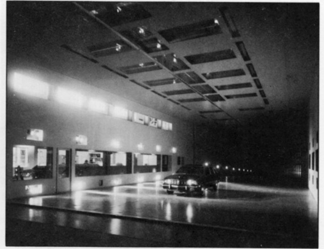
Figure 12 — Front view of test section, showing the floor boundary layer primary-intake-suction slot.
