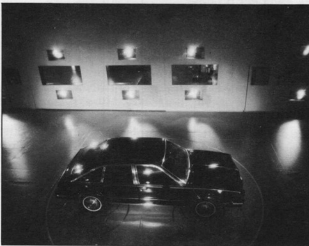
Figure 14 — Test vehicle mounted on the main balance turntable in the test section.
