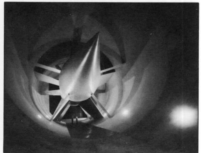
Figure 9 — Fan and tail cone of the motor nacelle.
