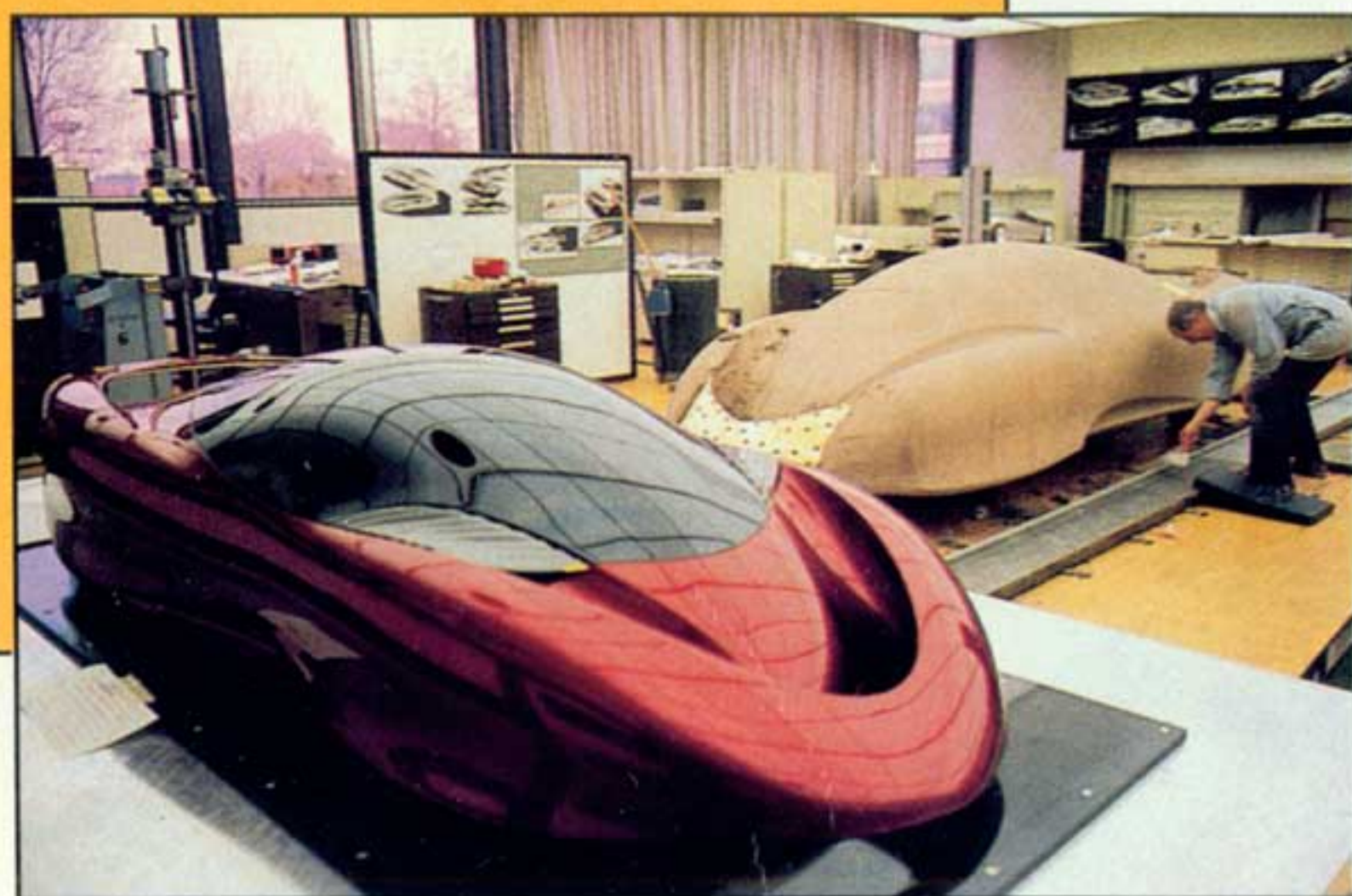
SRV-1 seating buck, top right, is surrounded by sketches of the then-named "Stealth." Sculptor works on clay, lower right, with scale model as guide.
